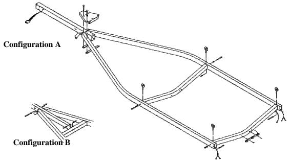
♦ In configuration A, line up the holes in the tongue, boom, boom to tongue plate and mounting straps and place in carriage bolts.
