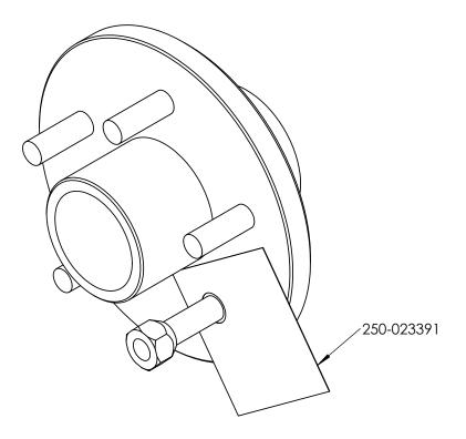
NOTE: DECAL 250-023391 NEEDS TO BE APPLIED TO EACH HUB OR DRUM ON ALL ASSEMBLED OR SEMI-ASSEMBLED TRAILERS BEING SHIPPER WITH THE TIRES REMOVED.
