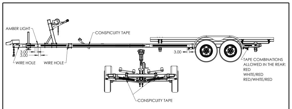
CONSPICUITY TAPE WILL BE SUPPLIED WITH ALL TRAILERS 10,000 GVWR AND ABOVE. APPLY THE TAPE TO THE REAR CROSSMEMBER, TONGUE AND BOOM. DUE TO THE VARIOUS CHASSIS LOCATIONS, IT WILL BE NECESSARY TO FIT TAPE AS NOTED ABOVE. TAPE MUST COVER AT LEAST 50% OF THE LENGTH OF TRAILER IN ALTERNATING COLORS.
