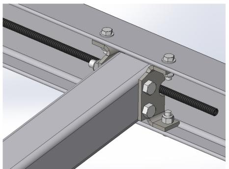
4) If the crossmember is mounted with hanger brackets without a wire cutout there are two routing options. The preferred method is to route the wiring under and around the crossmember and hanger brackets, as seen in the first picture below. The second option is to route the wire through one of the other hanger bracket holes, as seen in the second picture below. This route can become problematic if the crossmember height needs to be adjusted.
