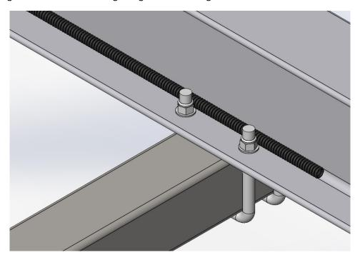
3) If the crossmember is mounted with hanger brackets check to see if the brackets have a wire cutout against the webbing of the I-Beam boom. If so route the wiring through this cutout as seen below.
