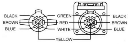
MOLDED TRAILER END As viewed from front face of 7-way connector with molded on cable. SEALED CAR END As viewed from front face of 7-way connector with sealed cable
